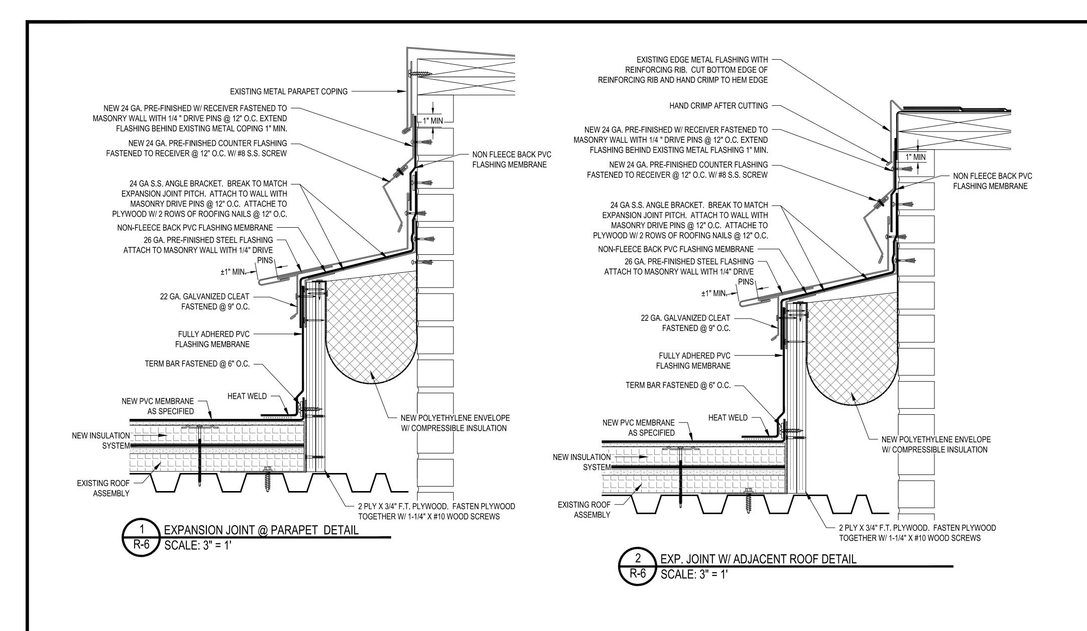
2 1/2" LAYER OF ISOCYANURATE INSULATION MECHANICALLY ATTACHED TO MEET MIN UPLIFT REQUIREMENTS PER FM GLOBAL. - 2 1/2" LAYER OF ISOCYANURATE INSULATION SET IN FOAM INSULATION ADHESIVE. 1/4" FIBERGLASS REINFORCED SILICON IMPREGNATED GYPSUM COVER BOARD SET IN FOAM INSULATION ADHESIVE - NEW ROOF MEMBRANE- AS SPECIFIED. **EXISTING METAL DECK**
